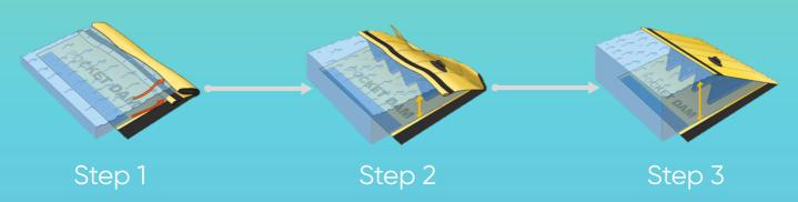
No site preparation needed prior to installation. Flow of water will automatically raise the pocket dam to inflated position.
